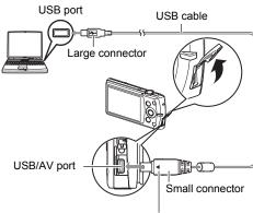
Making sure that the ◀ mark on the USB cable connector is towards the monitor screen side, connect the cable to the camera.
